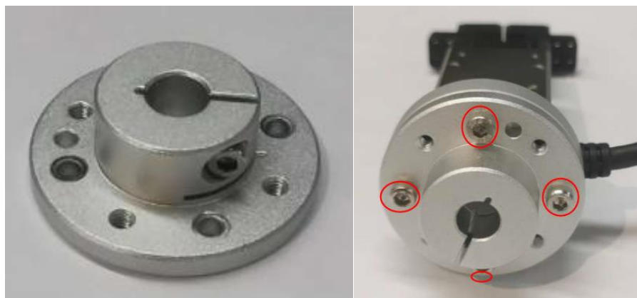
Figure 3.7 Install the end flange of MG400
