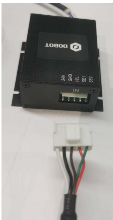
Figure 3.10 Connect gripper cable to control box
