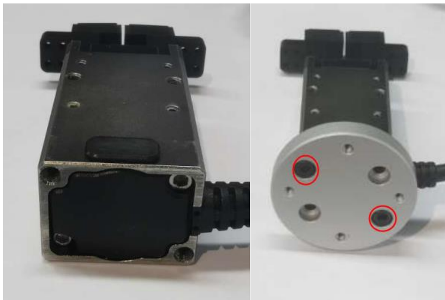
Figure 3.6 Install gripper mounting plate
