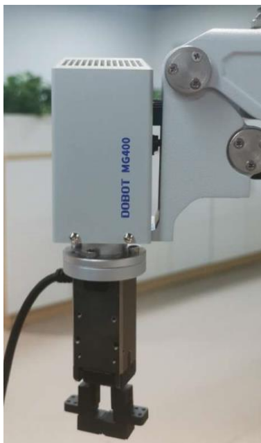
Figure 3.8 Install electromagnetic gripper
