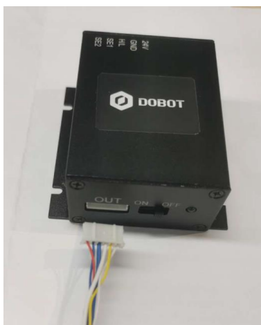
Figure 3.9 Connect electromagnetic gripper to control box
